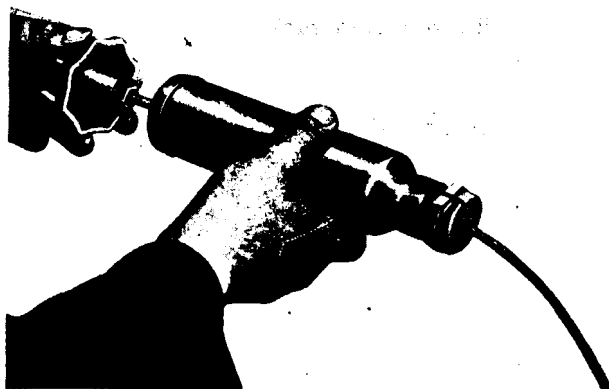
Fig. 174. Cable control inserted in a lubricating device
