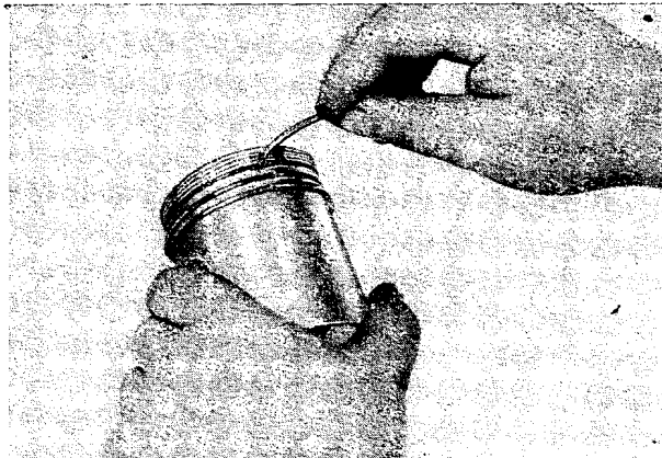
Fig. 40. Cleaning the ring grooves
